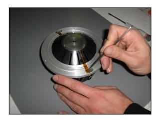
5. Unsolder the lead wires from the push button terminals
