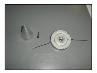
9. Pull out the diaphragm from the magnet structure
