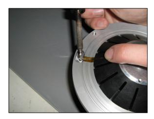
6. Unscrew the three small screws on the HF unit magnet assembly
