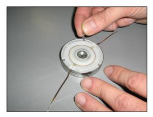
11. Fix the phase plug, screwing it on the HF magnet assembly
