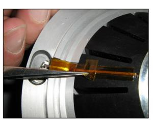
15. Solder the lead wires to the push button terminals
