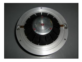
3. Remove the red varnish from the screws on the HF unit assembly using a soft cloth soaked in acetone
